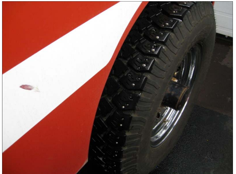
Above: specially-studded snow tires keep the Zamboni from slipping on its route. Below: The very organized Zamboni garage: a place for everything, and everything in its place.
